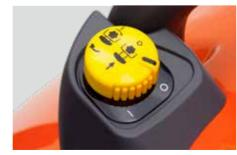
Electric-Over Hydraulic PTO Switch
